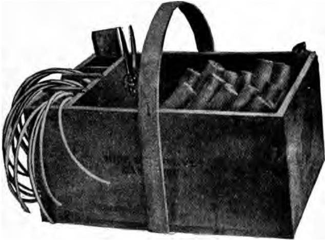
Fig. 15. A Handy Box for Carrying Explosives, Fuses and Caps. Compartments in One End Provide for the Caps and Fuses
